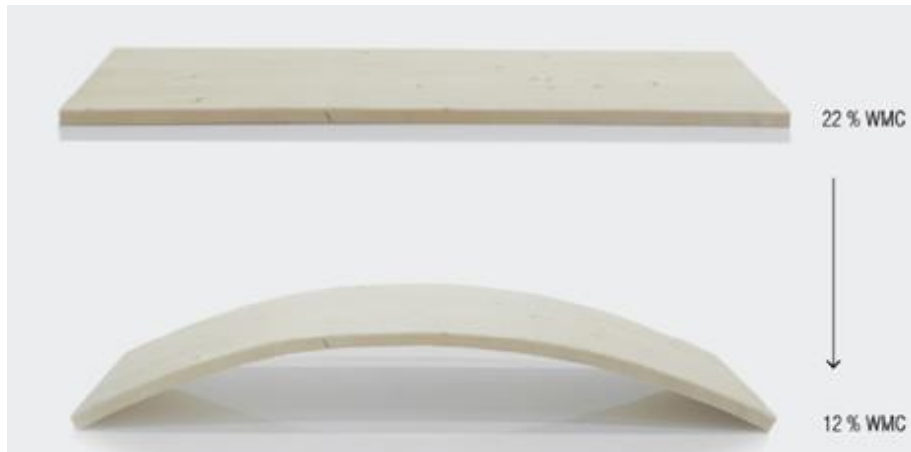
A two-layer bilayer wood panel bends during drying (WMC: moisture content of the wood).
