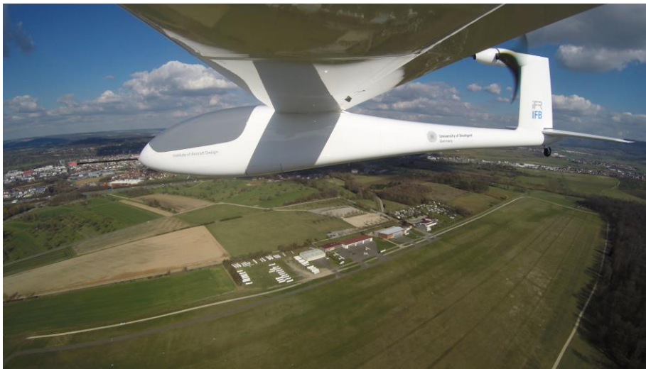
A scaled, unmanned electric aircraft of the type e-Genius. It is used to explore alternative propulsion concepts for energy-efficient and quiet aircraft. Photo: IFB/IFR/IAG
