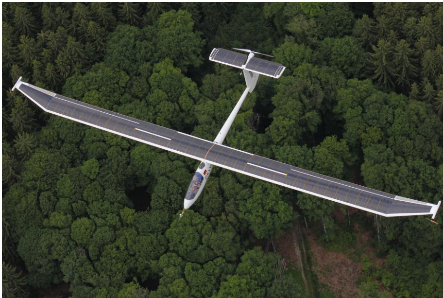
The experimental aircraft Icaré 2 during a test flight with electric wing end propellers.
