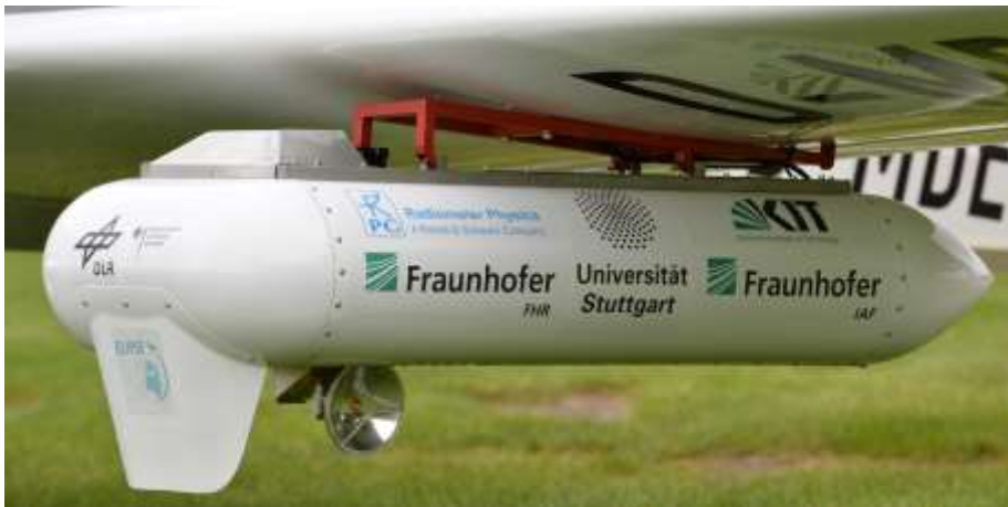
The E-band transmitter fitted to the wing of the exploratory aircraft. A small parabolic antenna ensures the correct alignment to the ground terminal. Photograph: Wolfgang Mies, Fraunhofer FHR
