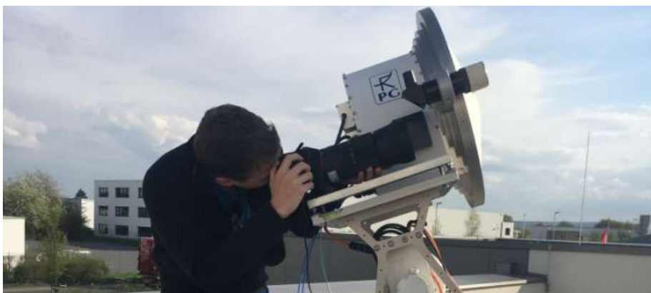
The receiving antenna on the ground is fitted with a tracking mechanism. Photograph: Parisa Harati, University of Stuttgart.
