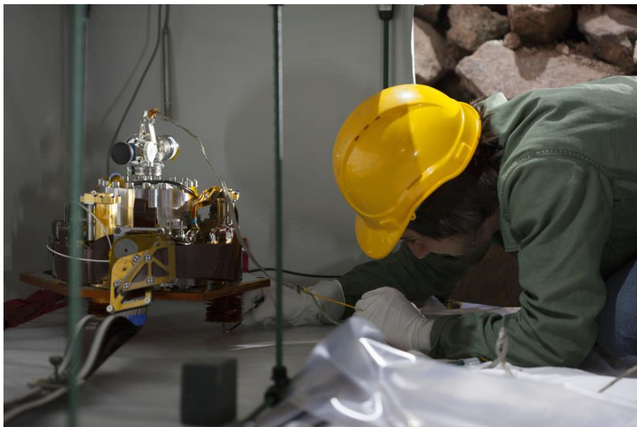
The SEIS instrument package during the installation in the test tunnel of the BFO, 110m below the earth's surface. Photo: Björn Oldsen
