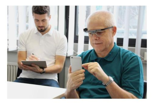
With eye-tracking glasses the visual movements of an older gentleman are recorded whilst he uses an app on a smart phone. The findings help the team at AGE-Ing. to improve the software. Photo: AGE-Ing.
