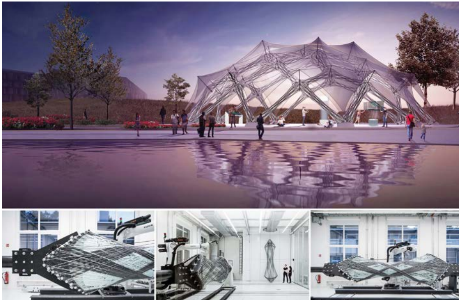
Visualization of the fiber pavilion and development of the additive manufacturing process in the research laboratory at the University of Stuttgart
