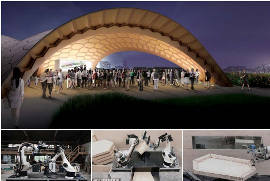
Visualization of the wooden pavilion and robotic platform for producing the load-bearing wooden elements.
