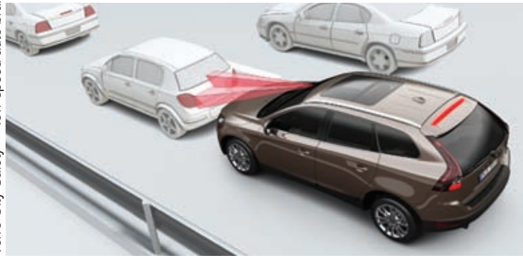
Volvo City Safety — low-speed auto brake
