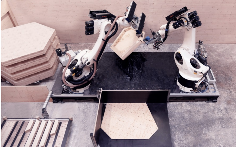
Die Mobile Robotic Timber Manufacturing Platform (TIM). Foto: ICD
