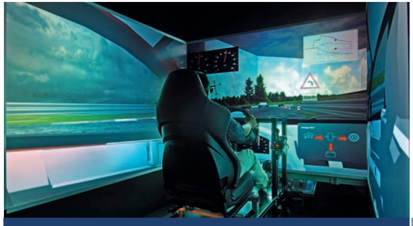
Implementation of the "virtual co-driver" in a static driving simulator for functional testing.
