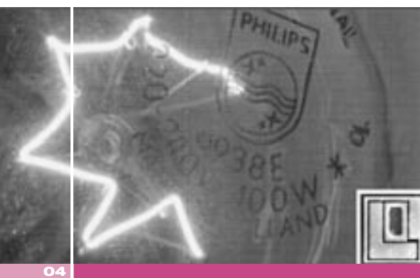
The impressively high dynamic range of 120 dB in this photograph results from both, a sophisticated logarithmic input stage in the underlying HDRC readout chip, and the six orders of magnitude in light-to-dark conductivity ratio of the a-Si:H based photodiodes on top of the TFC camera. The inset in the lower right corner presents a microscopic top view of one pixel.
