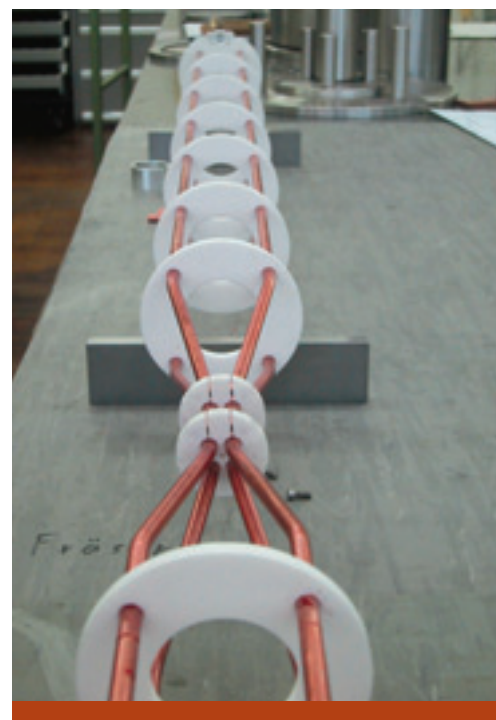
Magnetic wave guide for the realisation of a continuously pumped high-flux atom laser with chromium atoms. Instead of cooling the atoms step by step at the same position, the cooling steps are separated in space.
