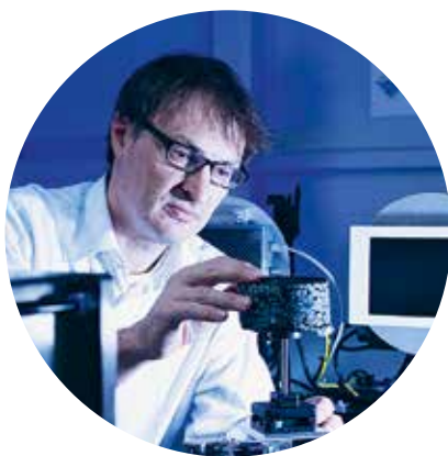
Holger Steeb prepares an asphalt sample for the X-ray tomography scanner.
