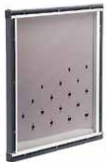
Façade demonstrator: The integrated flaps can be opened individually.
