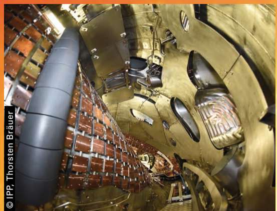
A view into the Wendelstein 7-X plasma container.
