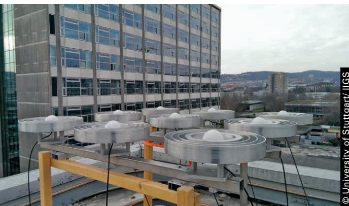
IIGS software permits low-cost upgrades of conventional, commercially available GPS equipment, which can then carry out millimeter-precise measurements.
