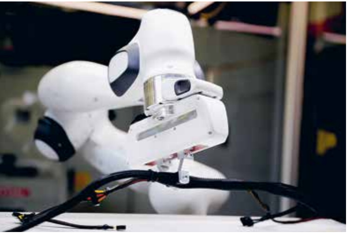
A glance at the work carried out at the ISW: With the aid of a software program, the aim is for the robot to learn to accurately locate and grasp an object, such as a cable.
