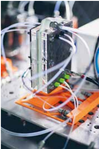
Research for sustainability: renewable energy is used to convert carbon dioxide into formic acid in the laboratory-based reactor.
