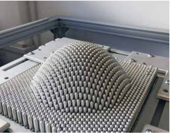
Modifiable geometry: the team is using the Dynapixel technology developed by their partner Cikoni GmbH for this purpose.
