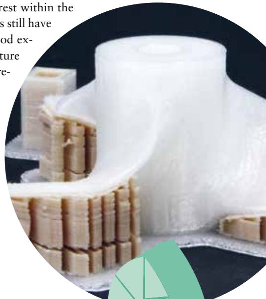
Biodegradable: a support structure made of salt and polymer
