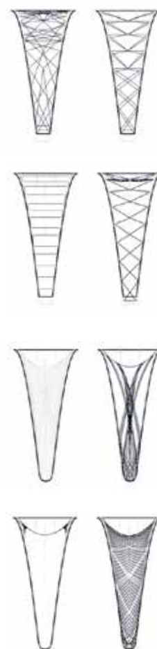
Unique funnel shapes: building with flax fibers requires a completely new design approach in the planning stage.
