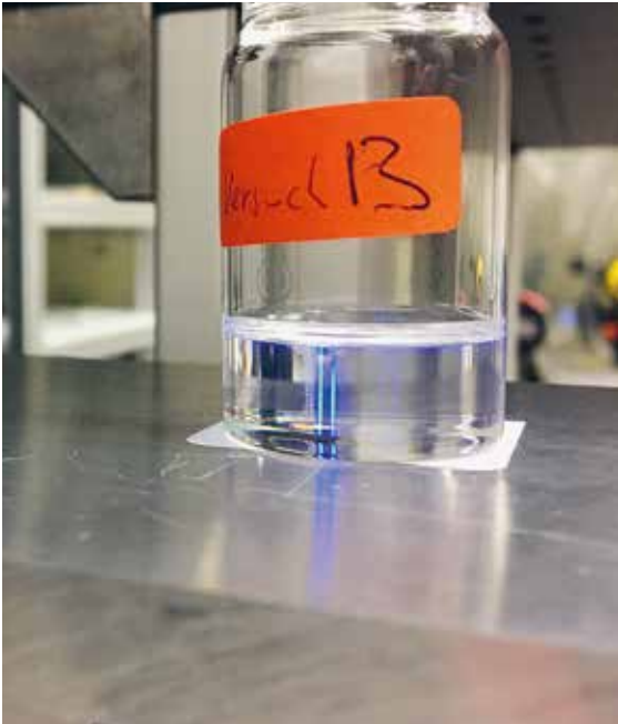
Left: Blue light caused by the two-photon polymerization effect in the resin basin at the Institute for Aircraft Design. Right: Good shape, thin walls – the surface quality can be improved at the IfW.
