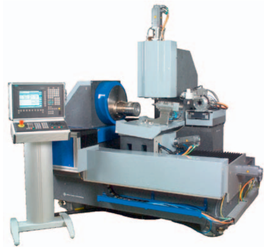
Fig. 1: Six-axis machine with an integrated optical measurement system (source: IPT, Aachen).
