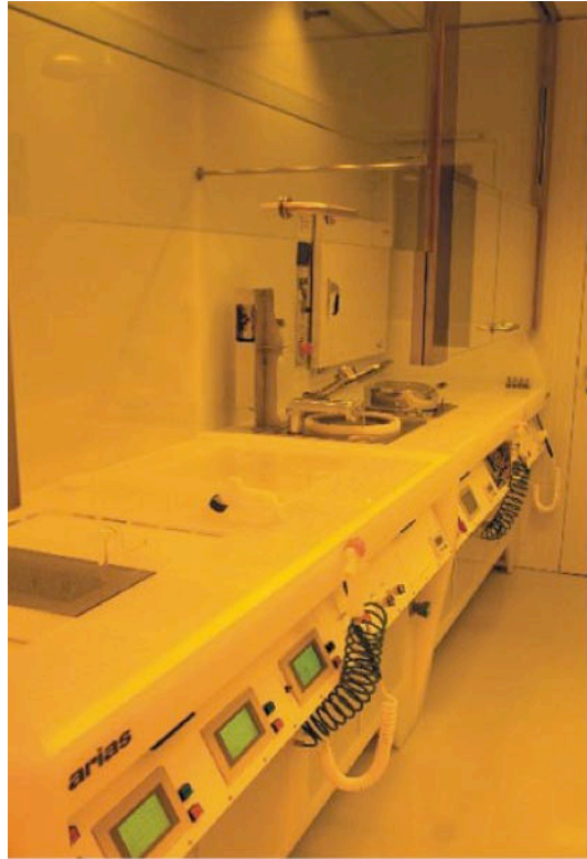
Fig. 1: Wet bench for the processing of substrates of up to 200 mm diameter and 20 mm thickness
