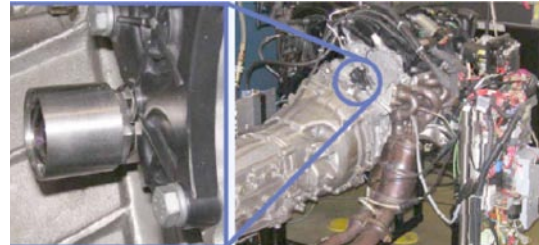
Fig. 5: Front piece of the hybrid endoscopic system attached to a test engine.
