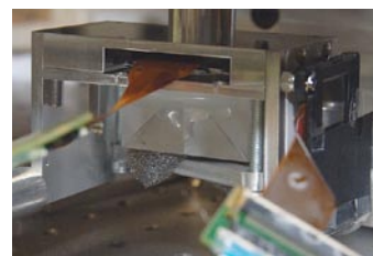
Fig. 4: The measurement head of a compact tomographic microinterferometer.
