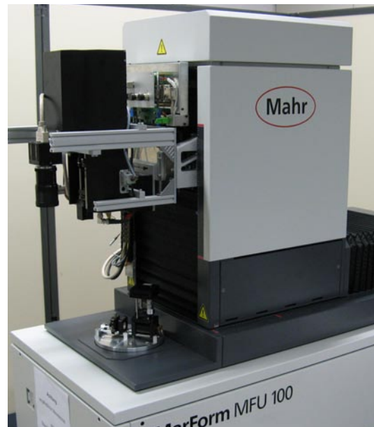
Fig. 2: Automated multi-scale measurement system based on a modified Mahr MFU 100.
