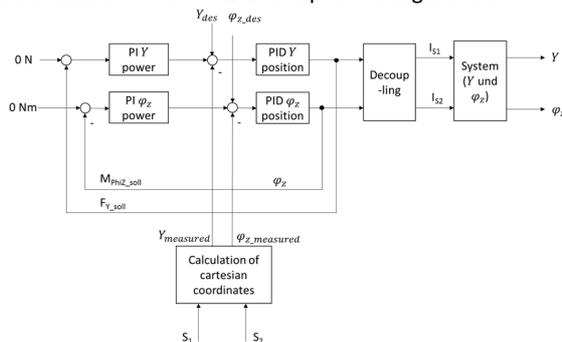
Figure 3. Control for minimization of the levitation power
