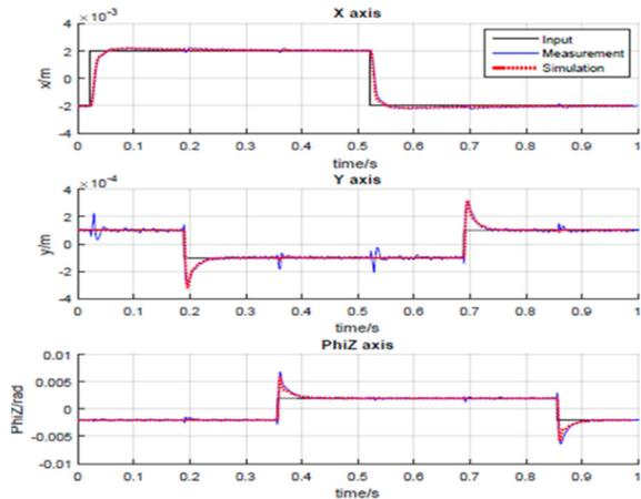
Figure 4. Step responses of the controlled axes
