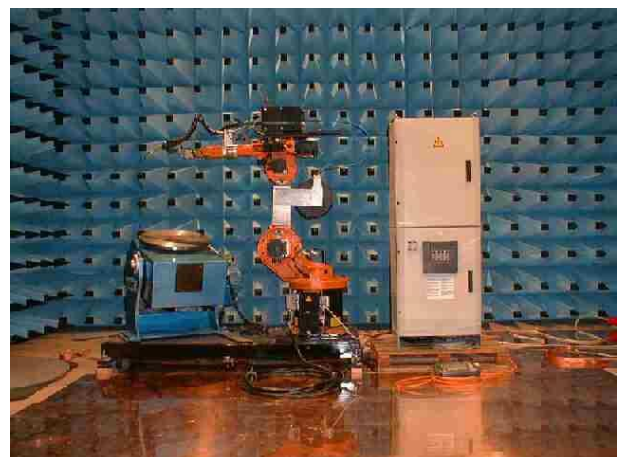
Fig. 7: EUT robot cell
